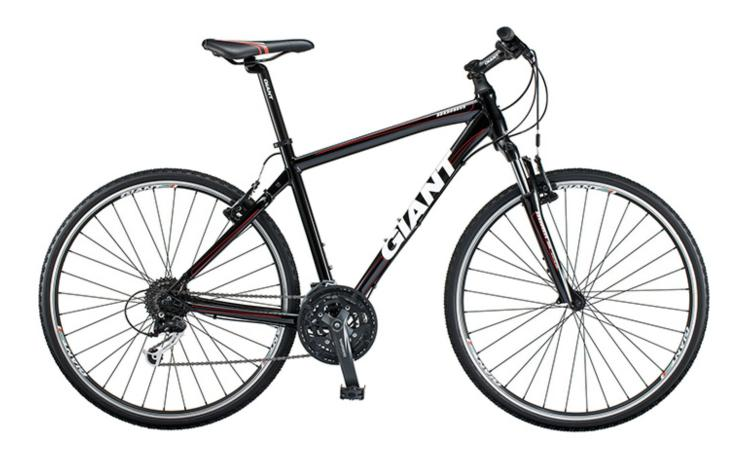
Strong and reliable aluminum frame with fast scrolling thanks to 700c wheels of diameter, perfect for long journeys. The bike has a front suspension to absorb ground movements rough surfaces. It can be locked for soft coverings.
